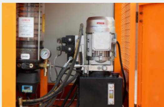
Automatic lubrication pump provides lubricating oil to seal plate
