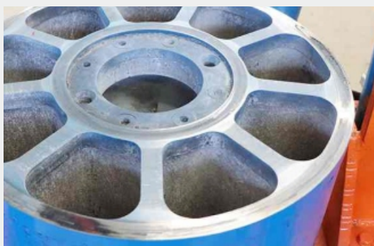
Sector hole rotor body, improving the volume of the rotor and decreasing friction area
