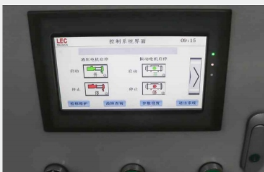
Touch screen operation panel for easy parameter setting
