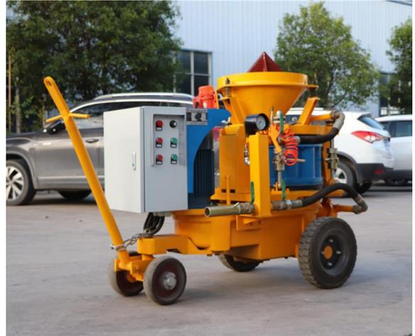
◆ Bag Cutter and Hopper with Vibrator/割包器、带振动器料斗
