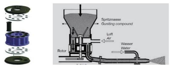
★ Rotor system could change different size rotor body, achieve different output capacity from 0.7m3/h to 3m3/h.
