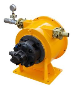
When the rotor unit drives single roller to rotate, hose is squeezed and deformed. After the roller rotate, the deformed hose recover by its elasticity. Thus the negative pressure in this hose is generated, sucking slurries, and discharging through output under rollers' push, finally forms pressure conveying of slurries.
