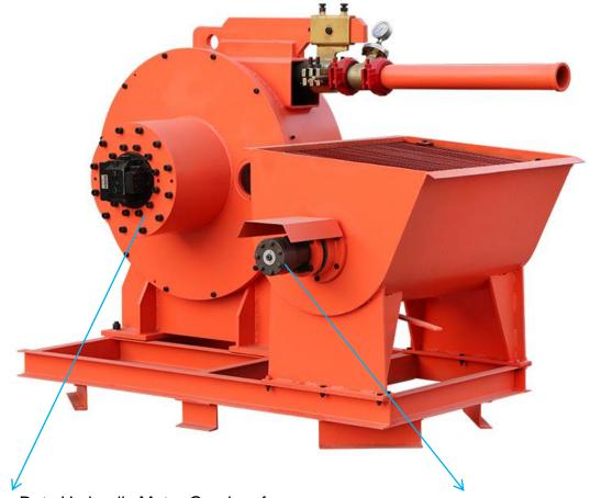
Heavy Duty Hydraulic Motor Gearbox for pump head
