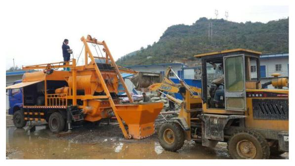
Trailer concrete pump with mixer used in vertical pumping
