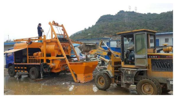
Trailer concrete pump with mixer used in vertical pumping
