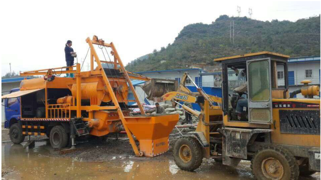
Concrete mixer pump in vertical pumping
