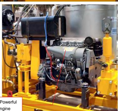
Deutz technology: Powerful air cooling diesel engine
