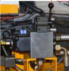
1. Grouting pump speed regulating valve:
