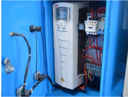
GH65 hose grout pump drive (ABB)
