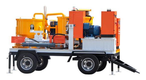
GGP400/1000/95/165DPL-E/A Grout Mixer and Pump are integrated with a screw feeder, mixing, agitator and horizontal hydraulic pump. It is mainly used to be made such as cement slurry or bentonite slurry, etc., for injecting in the sub-soil for soil consolidation, piling or even for long transport of material.
