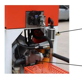
Adjustable output with this valve (LS control)
