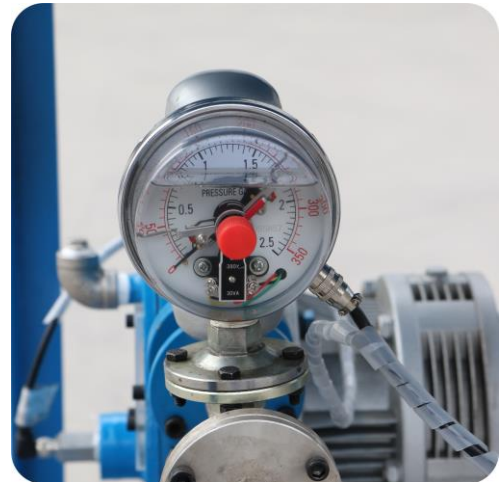
Electric contact pressure gauge
