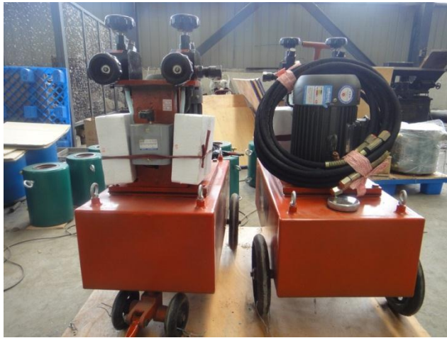
The photo of prestressing oil pump
